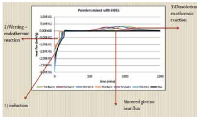
Figure 3. Calorimetry results showing the heat flux obtained on hydration of the materials tested with Hank's balanced salt solution (HBSS) which is a physiologic solution
